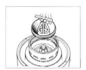
9. Use the inner hexagon spanner S=6 to remove the water distribution ring No. 29.
