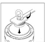
5. Use the drum body puller to separate drum part from the vertical shaft cone surface, and then lift the whole drum part.
