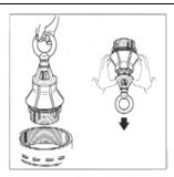
8. Use the drum body puller to lift the drum body No. 24. Use the valve seat dismantling tool to unscrew the plug, use the valve seat puller to pull the valve seat out, and use the valve core puller to pull the valve core out.
