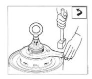
7. Use the piston puller to lift the piston No.21.
