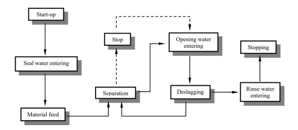
Note: The dotted procedure shall be implemented before stopping.
