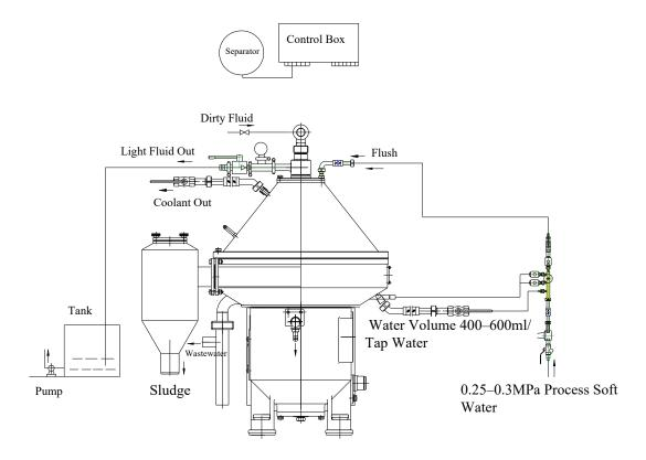
Feed pressure should be greater than 0.02 MPa. Use DN25 stainless steel ball valves. Be sure to slightly close the cooling water inlet valve.
