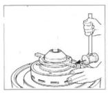
4. Use the small locking ring spanner install and tighten the small lock nut No.1.
