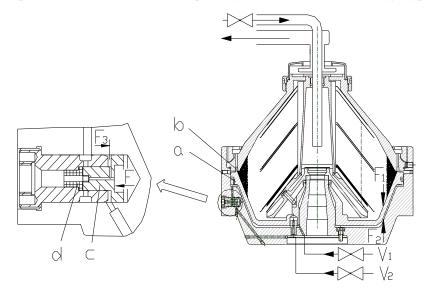
The cycle of residue removal comes to an end (normal separation is resumed):
