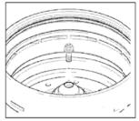
3. Use the socket wrench loosen the vertical shaft nut No. 10 (left hand threaded), and take it out.
