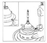
2. Use the screw plug dismantling tool to loosen screw plug of distributor No.18 (left hand threaded), and then remove the feed tube No.13 from the charge and discharge devices.
